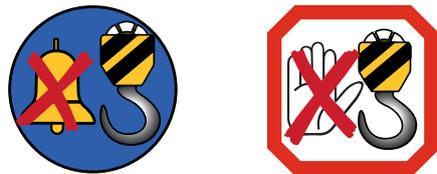
**OFF:** when operating with an inactive RCI / RCC limit, the indicator will have a cross on it.
