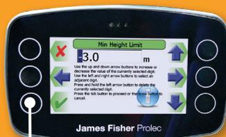
**1b** Enter a **known value** using the arrow keys and press the green tick to confirm.
