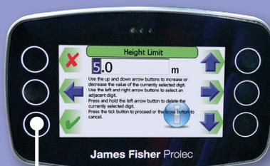
2b Enter a **known value** using the arrow keys and press the green tick to confirm.
