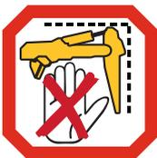
**OFF:** when operating without machine envelope control limits, the indicator will have a cross on it.
